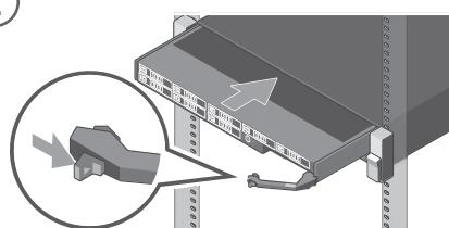
Beginning from the top, install the sled(s) into the enclosure.
